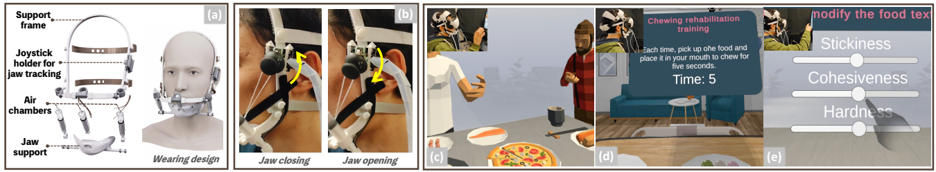
Figure 2: (a) On-Face Wearable Module. (b) Jaw Movement Tracking. Difference VR Applications for (c) Social Eating, (d) Healthcare and Rehabilitation and (e) Food Experience Design
